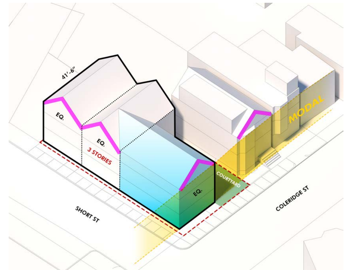
STEP 4: USE OF GABLE ROOF TO INTEGRATE THE NEW BUILDING WITH THE SURROUNDING CONTEXT. COLERIDGE ST FACADE IS STEPPED BACK TO MATCH EXISTING CONTEXT
